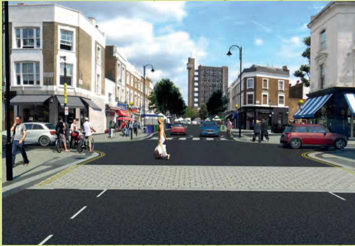
Raised table at junction to slow traffic
